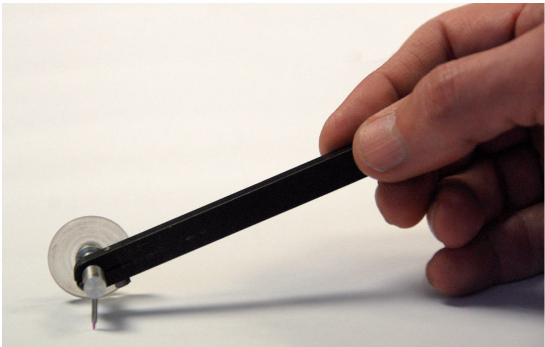
A straight line scribe. The small red protrusion at the bottom is the sapphire tip in its vertical cylindrical metal housing.
