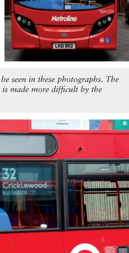
The built-in side blind box has been taken out of use and an 'e-ink' Kindle technology screen fitted inside the front lower deck window.
