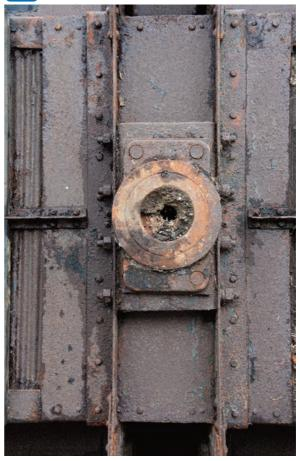
See Ref 93. The right-angle brackets bolted to the triangular plates continue all along the underside of the chassis to support the bogie roller on the other side. This photograph also shows the bogie pivots midway along the underside.
