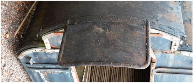
End roof strap, canopy fixings, various teak mouldings, upper and mid-level door runners (with the carriage lying on its side).
