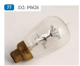
It is likely that tantulum incandescent lamps of this vacuum type were fitted, possibly with frosting on the outer half of the glass farthest from the bayonet fitting. *Source: Science Museum Group*
