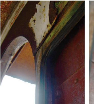
The four interior corners of a doorway end mirror frame, showing the inside of the exterior metal panelling, and reinforced plate with its bolts for the exterior door runner. The external teak flitched framework created a void between the inside of the metal panelling and the rear of the mirror glass.
