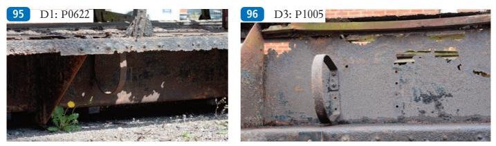
The looped strap in these images is probably one of two that held the auxiliary air reservoir tank in place. The righthand view from underneath shows a further set of four fixing holes to the right.
