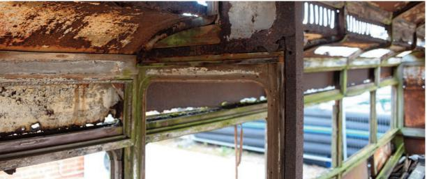
Detail of joinery at junction of advert frame above the window with the central draught screen. A void existed between the substantial wooden upper horizontal above the advert frame and the outer metal curve of the roof.
