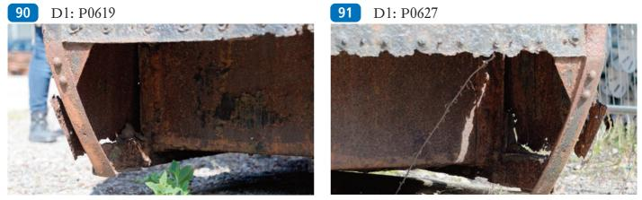
The 2-inch 'L'-shaped flitched verticals only had teak inserts above seat base level. These two photographs show threedimensional internal brackets connecting the curved 'L'-shaped vertical corner beams to the 3-inch upside-down lower horizontal beam.
