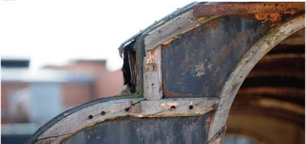
Bevel-edged moulding to doorway and ends of the carriage.
