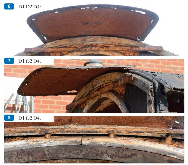
The overhead metal runner is clear of the teak mouldings and supported by six short horizontal metal posts secured from inside.
