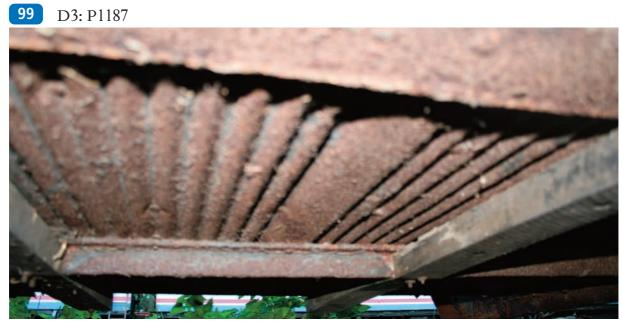
Taken when the carriage was at the Electric Railway Museum, this image shows the corrugated underfloor when it was is slightly better condition than in 2021. Source: Printz Holman.
