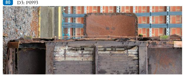
The underside of the canopy seen from below (with the carriage lying on its side).
