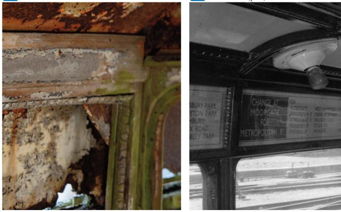
What held the front glass of the advert frames in place has not been established. Looking at one to the left (where it meets a central draught screen) there appears to be a closely spaced row of round studs around the edges, though these were not apparent elsewhere. See also Ref 110.
