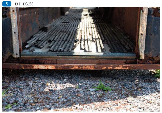
Floor slat end tread over lito-silo, also showing vertical teak moulding and lower door runner.
